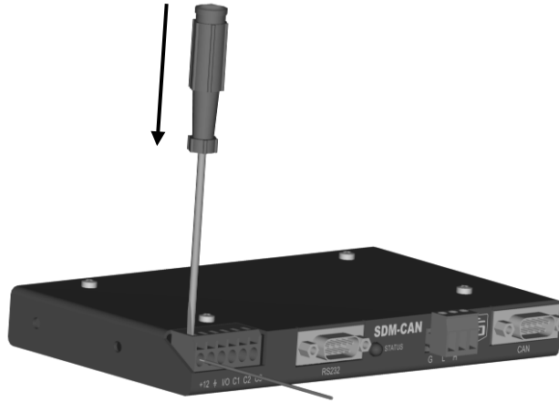
FIGURE 2-4. Using the Spring Loaded Terminal Blocks (Top Option)
